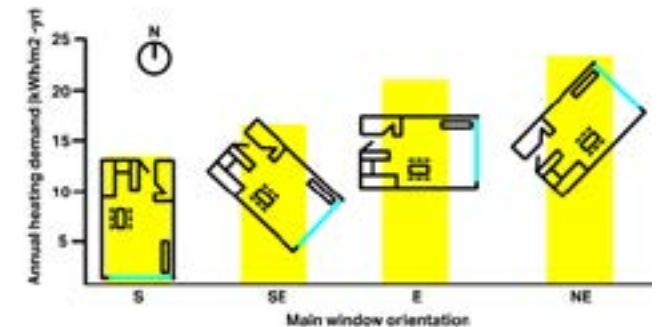
Figure 282: Building orientation influences the annual heating demand.
